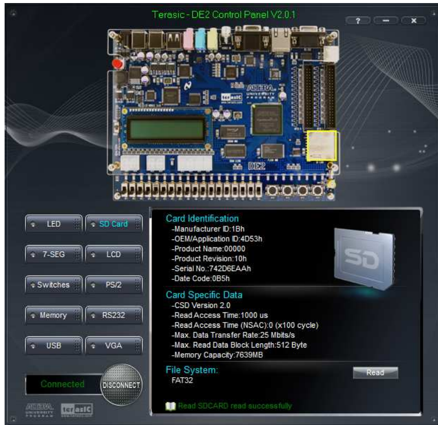
Figure 3.10. Reading the SD Card Identification and Specification.
