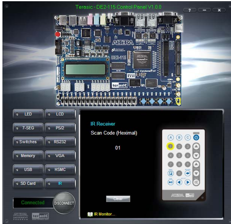
Figure 3-14 Testing the IR receiver using remote controller
