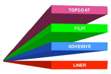
Figure 1. Construction of the high-performance labels for solar applications
