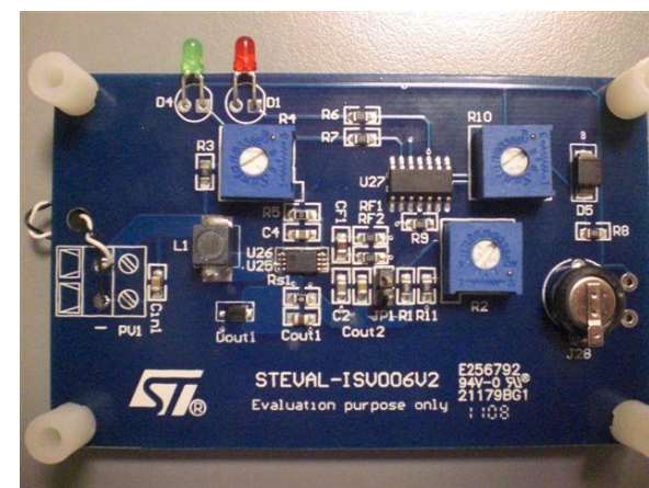
System evaluation board (STEVAL-ISV006V2 )
