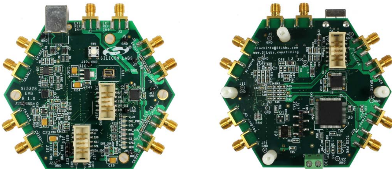
Top (U11 TCXO Plastic Cover Removed)
