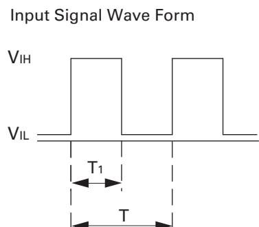
$V_{IH}=4.75V$  to  $5.25V$
