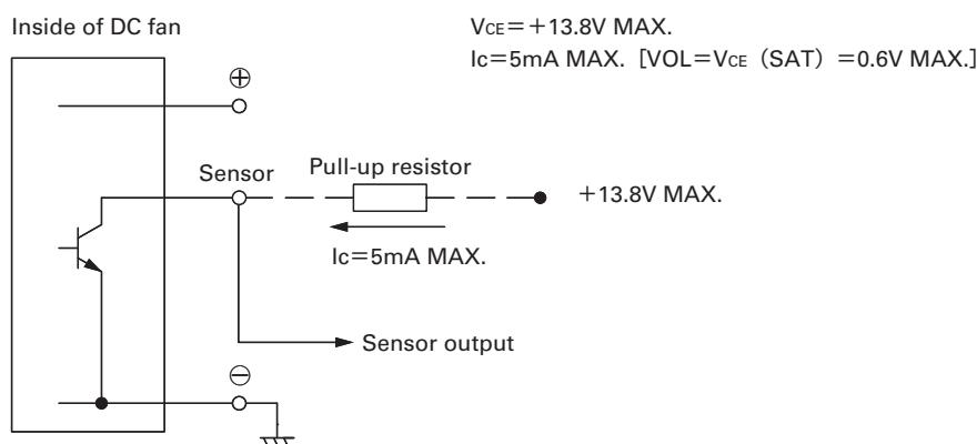
Output waveform (Need pull-up resistor)
