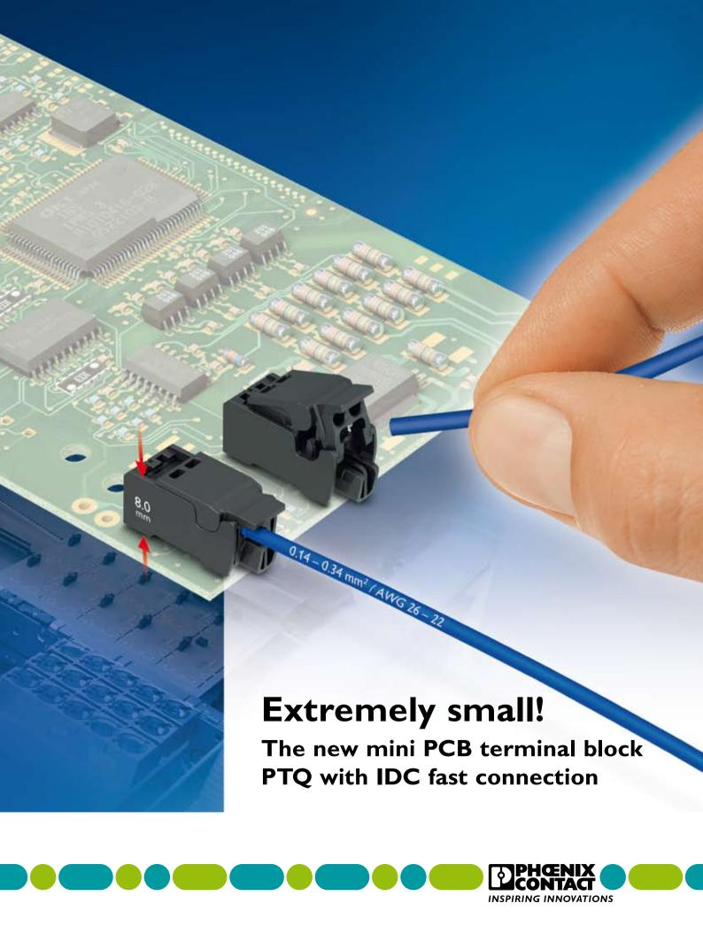
The two-position PTQ mini PCB terminal block with an overall height of only 8 mm was specially developed for use in THR soldering processes. The tape on reel packaged PTQ is suitable for fully automated assembly processes, enabling a time saving and increased production efficiency.
