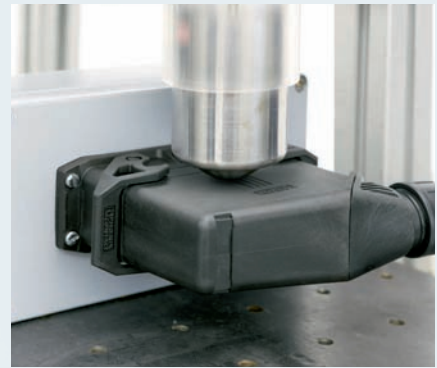
Impact of falling hammer weighing 1.7 kg
