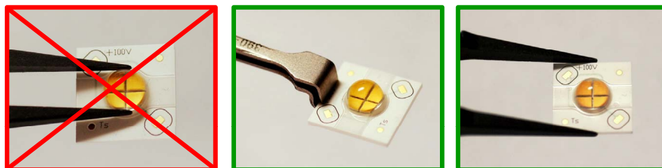
Figure 3. Incorrect handling (left) and correct handling (middle and right) of LUXEON H emitters.
