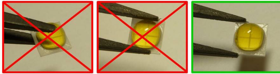
Figure 3. Incorrect handling (left and middle) and correct handling (right) of LUXEON M emitters.
