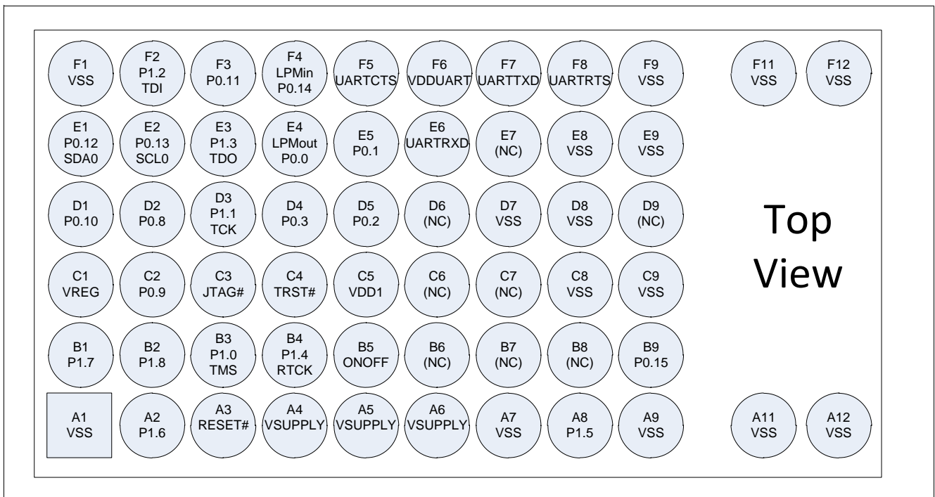
Figure 2 Pin Configuration for PAN1322-SPP in Top View (footprint)
