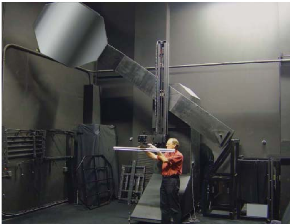
FIG. 1. LSI goniophotometer in the testing laboratory.
