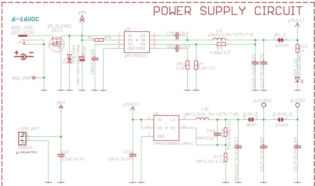
Note that the whole 3.3V part is not mounted (elements marked as NA) by default because we use the internal 3.3V DC-DC convertor in the iMX233. However, the internal DC-DC in the processor is not very reliable when a lot of current is required. It is better to mount the elements of the 3.3V part circuit if you wish to use 3.3V at heavier loads.
