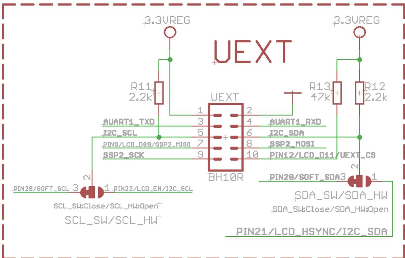
\*Note the two jumpers PIN29/SOFT\_SCL – PIN22/LCD\_EN/I2C\_SCL, and PIN28/SOFT\_SDA3 – PIN21/LCD\_HSYNC/I2C\_SDA which by default are set to a software SPI. They can be used to set the whole UEXT to a hardware SPI.
