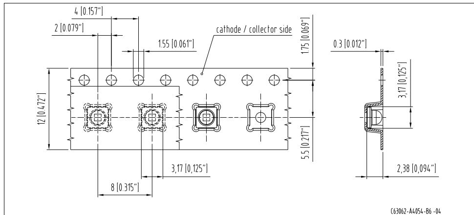
**Tape and Reel<sup>5)</sup> page 21****Gurtverpackung<sup>5)</sup> Seite 21**12 mm tape with 600 pcs. on  $\varnothing 180$  mm
