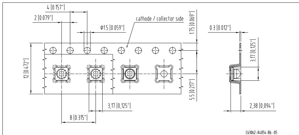
**Tape and Reel<sup>5)</sup> page 24****Gurtverpackung<sup>5)</sup> Seite 24**12 mm tape with 600 pcs. on  $\varnothing 180$  mm
