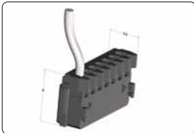
Unstripped wires inserted into MT housing.
