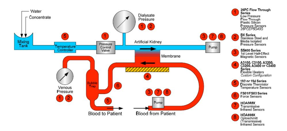
Note: Value propositions have been provided for flexible heaters, force sensors, Hall-effect magnetic position sensors and pressure sensors.
