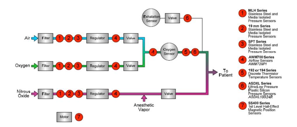
Note: Value propositions have been provided airflow sensors, Hall-effect magnetic sensors and pressure sensors.
