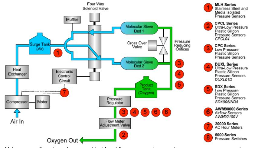
Note: Value propositions have been provided for airflow sensors, hour meters, pressure sensors and pressure switches.
