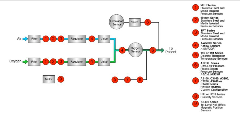
Note: Value propositions have been provided for airflow sensors, flexible heaters, humidity sensors, Hall-effect magnetic sensors and pressure sensors.
