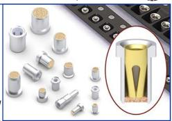
ly been screen printed on pads adjacent to the holes) and the board is reflowed in the same pass as other SMT components. Solder will fill the plated through-holes and achieve solder joints as reliable as wave soldering. The OFP® barrier prevents solder paste from being picked-up inside the contact during pick in place assembly. "Overprinting" paste on the solder mask can be used to adjust the volume of paste required to fill each hole.
