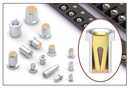
hole components to be placed simultaneously with surface mount parts on pick-'n-place assembly lines – eliminating the need to hand place the receptacles in an additional manufacturing step. The OFP® barrier permits the sockets to be vacuum picked from the tape prior to placement in a hole in the circuit board.
