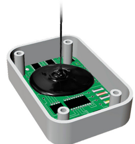
Example of potting for UL913 compliance
