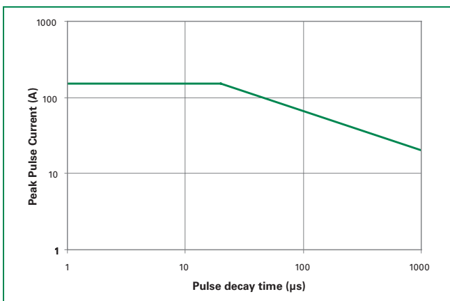
Figure 1: Non-repetitive Peak Pulse Current vs. Pulse Time
