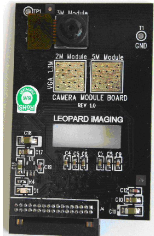
Figure 10. 3M Camera Board
