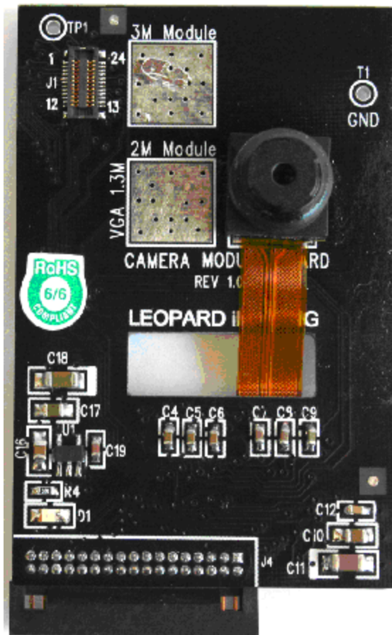
Figure 11. 5M Camera Board
