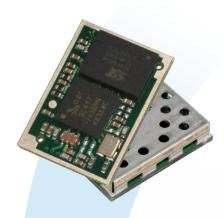
The BTM430 and BTM 431 Bluetooth® modules from Laird Technologies have been designed to meet the needs of developers who wish to add robust, short range Bluetooth data connectivity to their products. They are based on the market leading Cambridge Silicon Radio BC04 chipset, providing exceptionally low power consumption with outstanding range.
