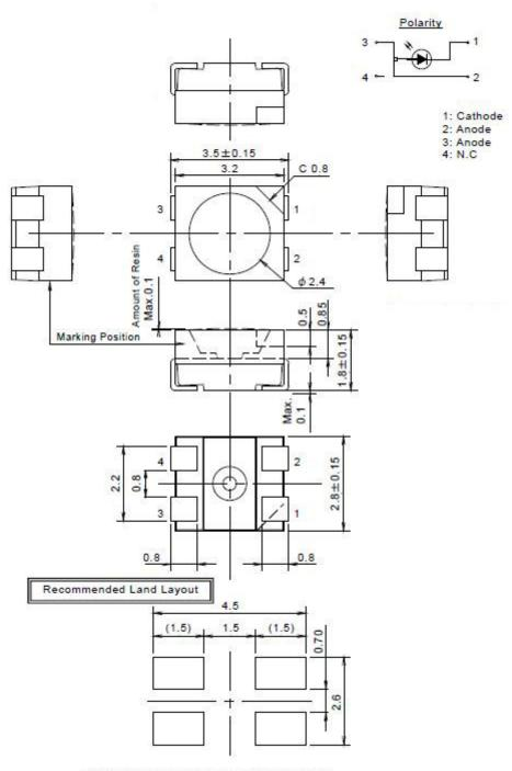
(Note1) Tolerance unless specified: ±0.1 mm.
