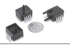
The pressure is on. The answer is here. No matter the need, Honeywell Sensing and Control (S&C) has the microstructure, plastic pressure sensor solution. Our sensing element design consists of four piezoresistors galvanized with a thin, chemically etched silicon diaphragm. A pressure change will flex the mechanism, causing a strain in the diaphragm and the buried resistors. The resistor values will change in proportion to the
