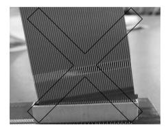
Do not insert the FPC diagonally. Doing so will result in the corners of the FPC catching on the contacts and will cause deformation of the contacts.
