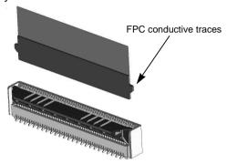
3 Press down the actuator in the direction shown.
