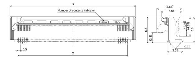
Note 1: The coplanarity of each terminal lead within specified dimension is 0.1 mm Max.
