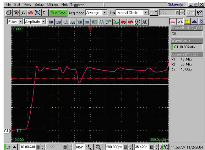
Figure 17. TDR impedance measurement screen.
