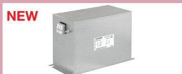
FMAC SINE: Sine wave output filter, allows motor cables up to 200m under full load. 4-16A, 500/288 VAC, screw clamp terminals
