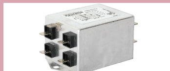
FMW4-65: Compact filter for three phases, neutral conductor and ground, 3-20A, 250/440 VAC, quick connect terminals
