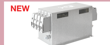
FMBD NEO: Terminals for 3 phases, neutral conductor and ground, intended for use in 4 wire systems. 8-200A, 300/520 VAC, screw clamp terminals
