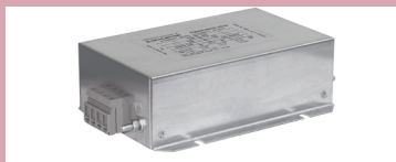
FMAD: High current filter w/neutral conductor, approved for high temperature applications, 6-550A, 275-480 VAC, screw clamp terminals
