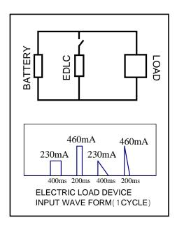
EDLC in parallel connection with battery\* can stabilize the battery load charge.
