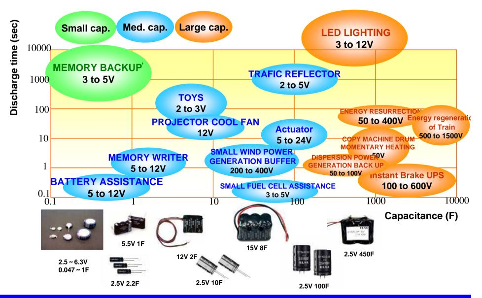
Features & Benefits of Electric Double Layer Capacitor (compared to battery)
