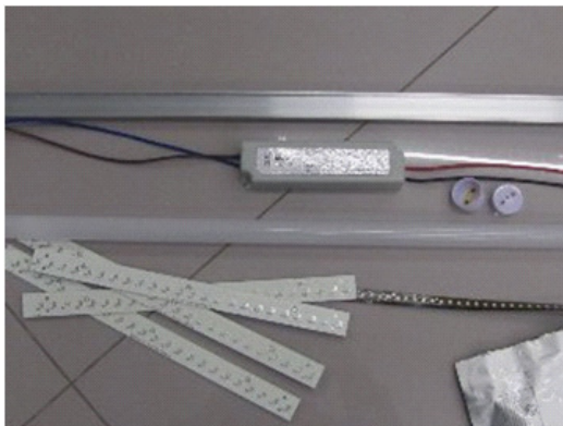
Figure 10: Parts used to assemble the prototype T8 lamp
