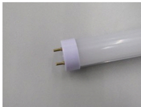
Figure 13: Tube end caps used to secure the assembly
