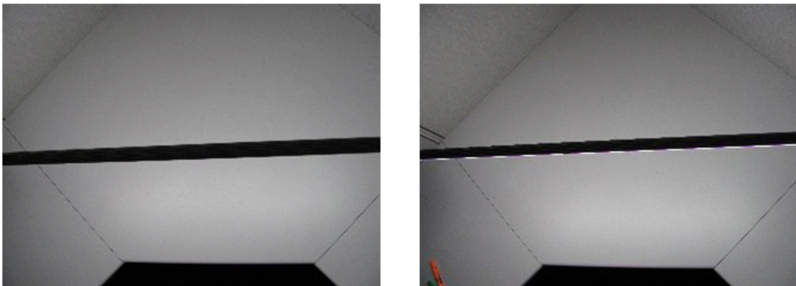
Figure 17: Visual performance of prototype T8 lamps in typical office cubicle work area, viewed from above (left: 96-LED T8 lamp, right: 60-LED T8 lamp)
