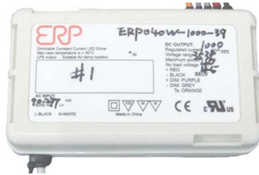
Figure 4: CXA2530 retail track light driver
