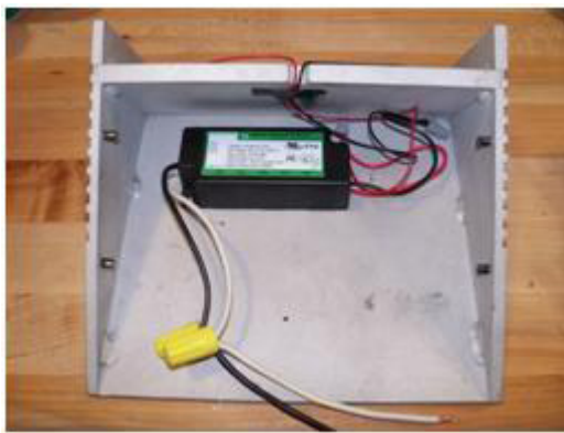
Figure 15: Driver for XP-G prototype sconce
