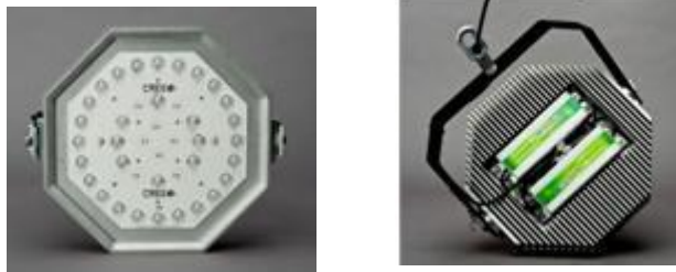
Figure 17: Assembled XM-L prototype high-bay luminaire
