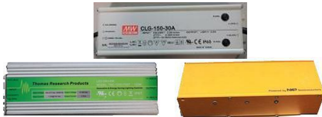
Figure 11: Power supplies (left: Thomas Research, right: NXP)
