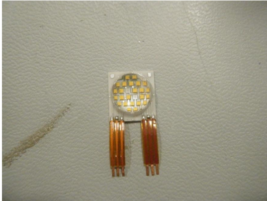
3-conductor ribbon cables soldered to the XLamp MP-L pads
