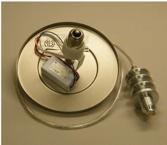
Figure 13: LED-drive electronics secured in ceiling receptacle cover
