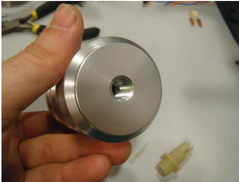
Heat sink has been tapped for strain relief.
