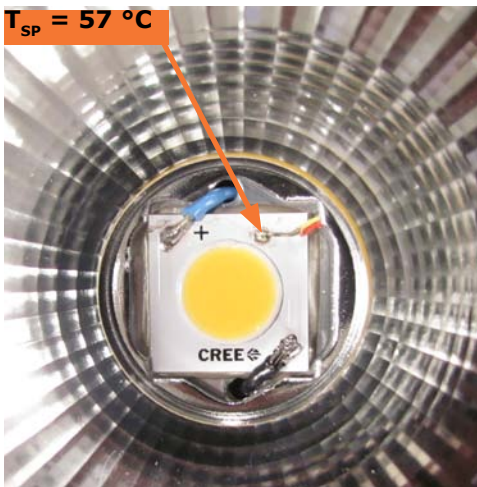
Figure 9: CXA1507 PAR30 T_{SP} measurement with thermocouple
