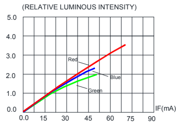
FIG.2 RELATIVE LUMINOUS INTENSITY VS. FORWARD CURRENT
