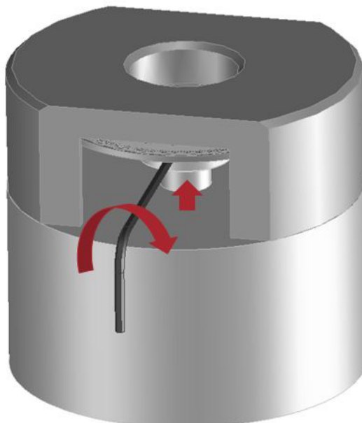
Figure 1d. Tighten the set screws
