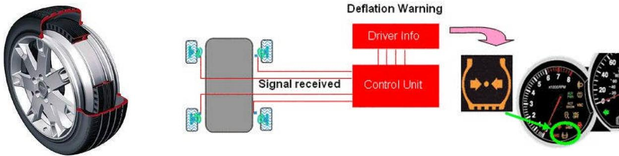
Figure 1: Tyre pressure monitoring system block diagram
