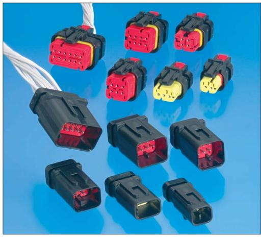
The AMPSEAL 16 Receptacle and Pin housings come fully assembled, offering a one-piece approach for applied cost savings. Receptacle housing assemblies consist of the plug housing with both interface and wire seals, wire seal cover, TPA, & CPA.
