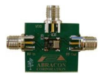
To facilitate quick engineering evaluation of the Frequency Translators, Abracon also offers Evaluation Boards – with either the 20MHz or 40MHz Translators already mounted for ease of use. Designers can input a 10MHz reference into the Evaluation Board and quickly characterize the output characteristics of the Translator solution.
