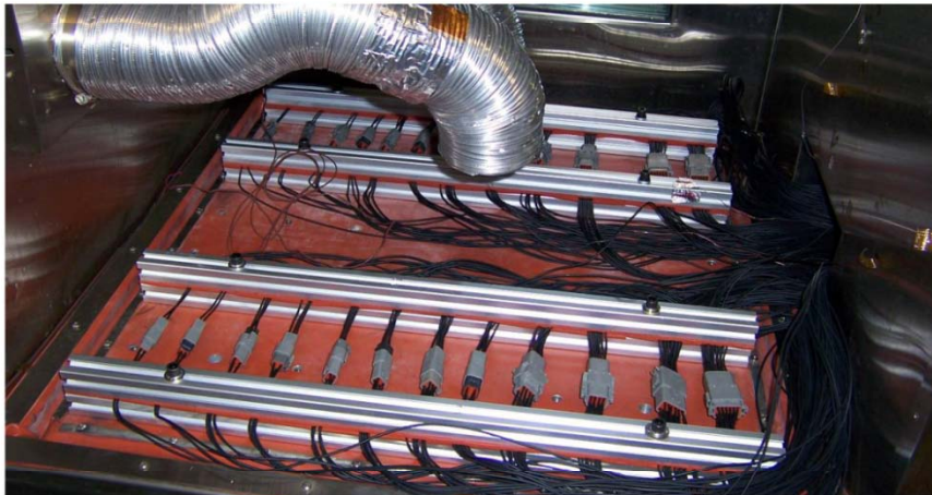
HALT samples 1 to 24 in chamber. Cold Step Stress, Hot Step Stress, Rapid Thermal Cycling.
