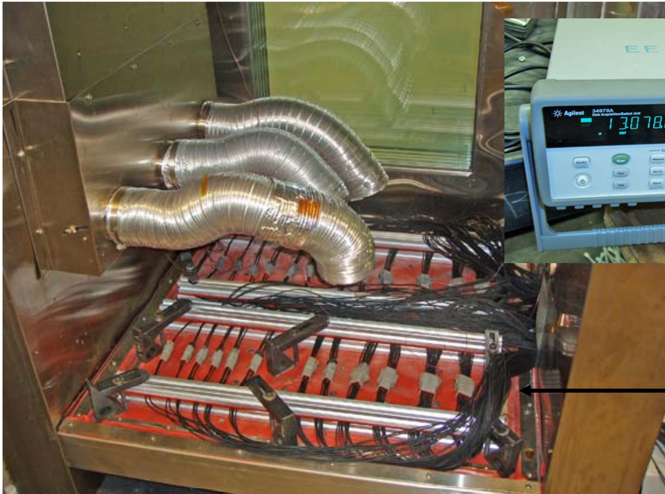
HALT samples 13-24 in chamber. Vibration Step Stress, Combined Environment.
