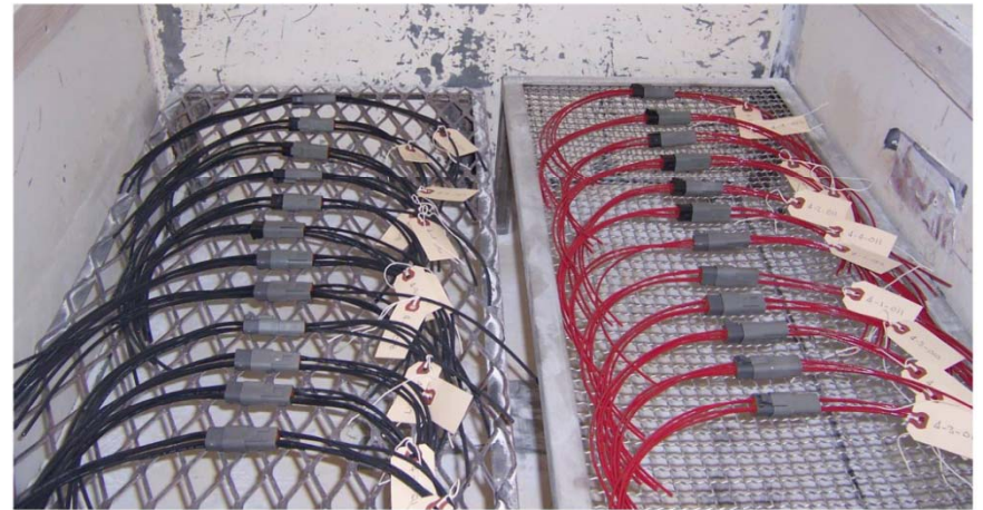
Dust Testing – 4 position samples
