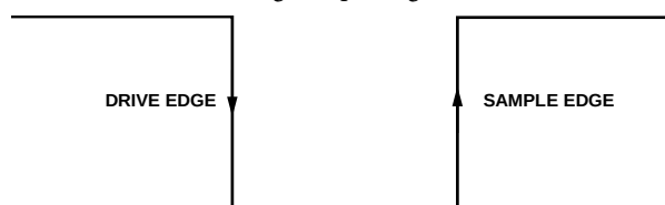
Figure 25. SPI Mode 3 SCLK Edges
