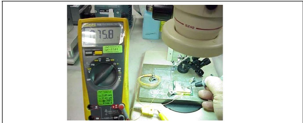
Figure 5-9. Applying the Adhesive on the Thermocouple Bead
