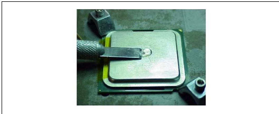
Figure 5-12. Filling the Groove with Adhesive
