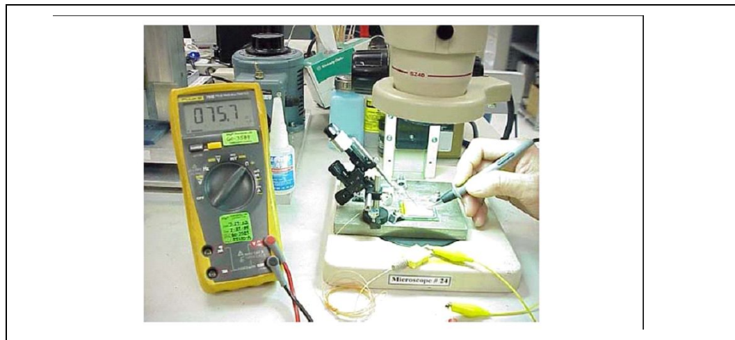
Figure 5-8. Measuring Resistance between Thermocouple and IHS
