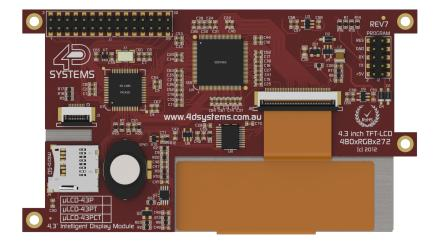
Audio support provided on the display module is supplied by the **PICASO** processor, an on-board audio amplifier and  $8\Omega$  speaker. A simple instruction enables the user to play audio files while continuing the execution of the user application code, such as display updates, touch recognition, communications and much more.
