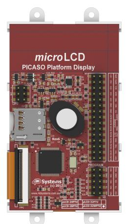
The μLCD-32WPTU has a 3.2" Wide TFT LCD display at the forefront of the design that showcases the power and capabilities of the PICASO processor. Combining a resolution of 240x400 pixels with 65K True to Life colours, the display module is perfect for animations, slideshows and other multimedia presentations.
