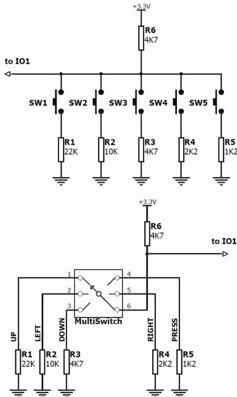
Unused buttons do not need resistors to be connected to the circuit. Table below lists the buttons and corresponding resistor values.
