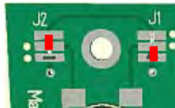
Solders pad J_1 and J_2 connection for reversed heat flux direction
