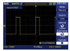
Monitor and analyze long-term signal behavior by recording data continuously over an extensive period of time and playing them back for post acquisition analysis. Data is recorded in a sequence of up to 2500 frames.
