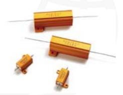
The AHA series is high power resistors housed in a very strong aluminum case. The sides of the aluminum case are corrugated for added strength. The resistors offer power ratings up to 250W, and are available in a tolerance as narrow as 0.25%.
