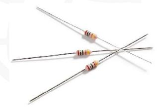
The Yageo HHV series resistors are made of metal glaze film, with tinned connecting leads of electrolytic copper welded to the end of caps. This series is also very humidity-resistant.
