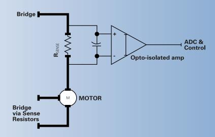
The important attributes in this case are the availability of values below 10m, up to 5W power rating with good surge withstand ability and low inductance. The ideal choice for RMS phase currents up to about 20A is the OAR series, which is a pluggable, formed tape element resistor available in 1, 3 and 5W ratings. The 1W type is also
