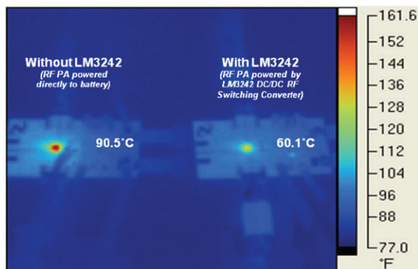
LM3242 reduces PA heat by 30°C at maximum RF power (28 dBm).
